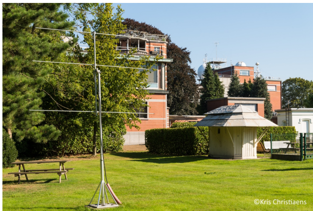
Figure 8 – Receiving antenna at the BRAMS station located in Uccle. It is a 3-elements Yagi antenna set up vertically.
