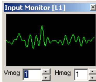
If the signal color is mostly red, decrease the audio gain of the line-in entry in the volume control panel of Windows.
