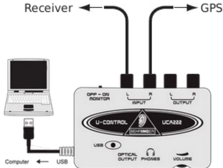
Connect the receiver to the left RCA input of the audio interface with the help of the RCA-RCA cable and the Jack/RCA adapter provided by BISA. Connect the GPS to the right RCA input.
