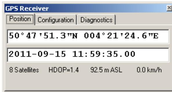
The dialog box should display the current GPS position and UTC time. High accuracy is achieved when the number of satellites is close to twelve and the HDOP value is close to one.
